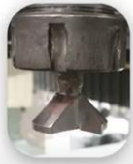
45° upcut end milling cutter
